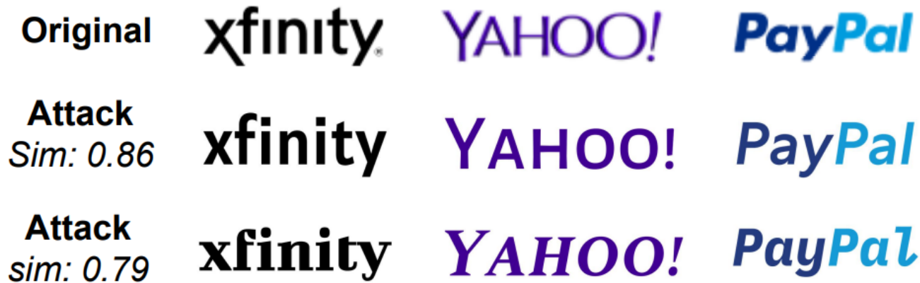
Figure 4: Text Logo Attack Examples —The first row displays the brand’s original logo. The second row shows attack fonts with cosine similarity (about 0.86) that is slightly below the detection threshold. The third row exhibits adversarial logos with a lower cosine similarity (about 0.79). All these fonts can bypass detection.
